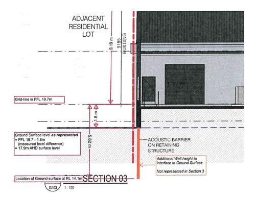
The existing surface is represented as being only 1.8m below the FFL line of 19.7m. That is, the natural surface level at the Lot boundary on drawing DA08 Section 3 is measured as approximately RL17.9m.
