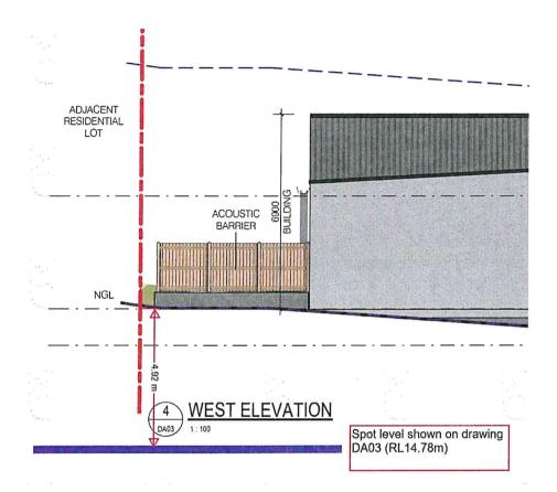
It appears that the long sections on drawing DA08 and DA07 do not present the natural surfaces at the western Lot boundary and the interface between design levels and natural surface levels correctly.
